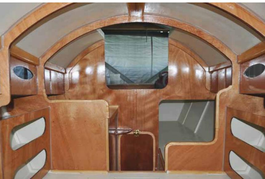
NIS 18 interior looking aft. Note galley on starboard side, quarter berth on port. Porta Potti is located behind door in centre of boat, and under cockpit sole. It is designed to be put out in the cockpit at night.
